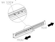
2) Fix the slides to the rack using M6 round screws and clip nuts.
