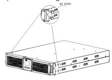
5) Slide the UPS into the rack and screw it as indicated with 2 x M6 screws and 2 x M6 nuts.
